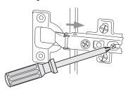
Turn screw as shown, to adjust the door position
