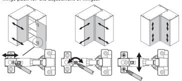
Turn screw as shown to adjust the door position.
