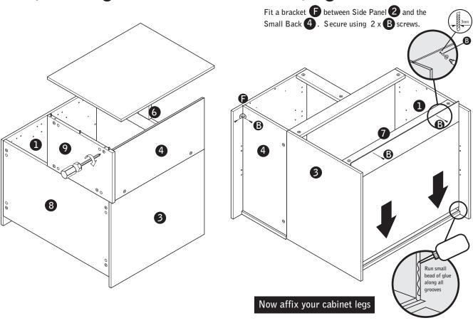
Slide the Back Panel into the groove.
