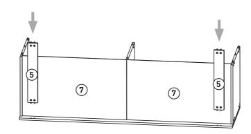
If you are using this cabinet for an integrated fridge / freezer, you should leave out panels (4) and (7), during the construction process.
