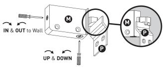
Ensure the front face of the unit is vertical by using a spirit level.
